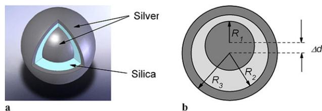
**Fig. 1** (a) 3D illustration of silver–silica–silver MNS. (b) Dimensions of an  $R_1$ – $R_2$ – $R_3$  silver–silica–silver multilayer nanoshell with core offset  $\Delta d$
