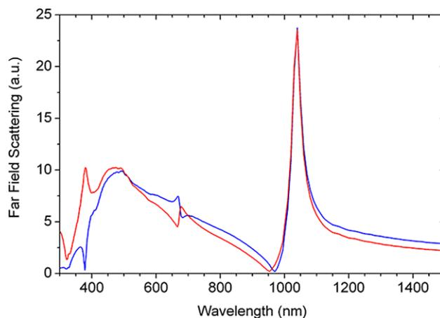
**Fig. 2** Far-field backward scattering (blue) and forward scattering (red) for 50–66–75 nm MNS. The symmetric dipole resonance can be seen in the vicinity of 1038 nm. Asymmetric quadrupole resonances are seen around 390 and 670 nm; the forward and backward scattering profiles in these vicinities are typical of Fano resonances
