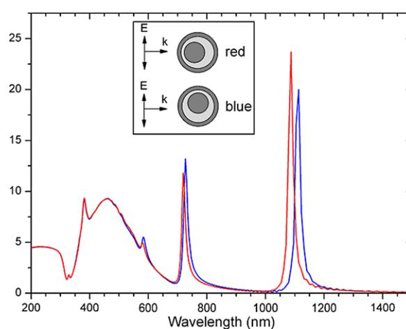
**Fig. 7** Extinction spectra for 50–66–75 nm MNS with different particle orientations. *Red curve*: incident electric field is polarized perpendicular to axis of symmetry. *Blue curve*: incident electric field is polarized parallel to axis of symmetry
