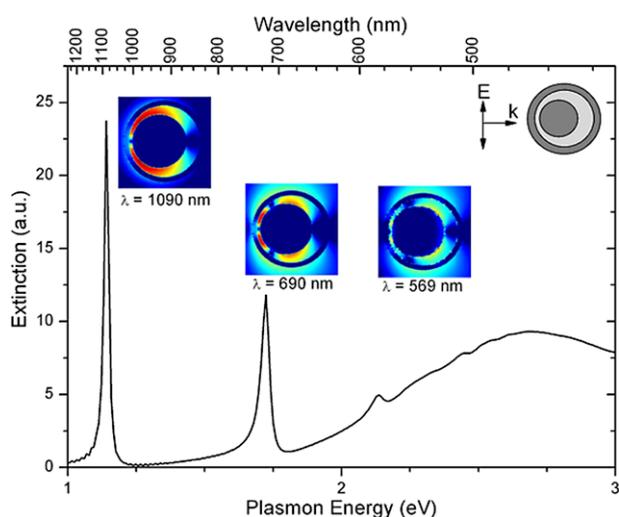
**Fig. 6** Extinction spectrum and field distributions for 50–66–75 nm MNS with  $\Delta d = 10$  nm. The hybridized natures of the quadrupole and octupole modes are seen in the field distributions
