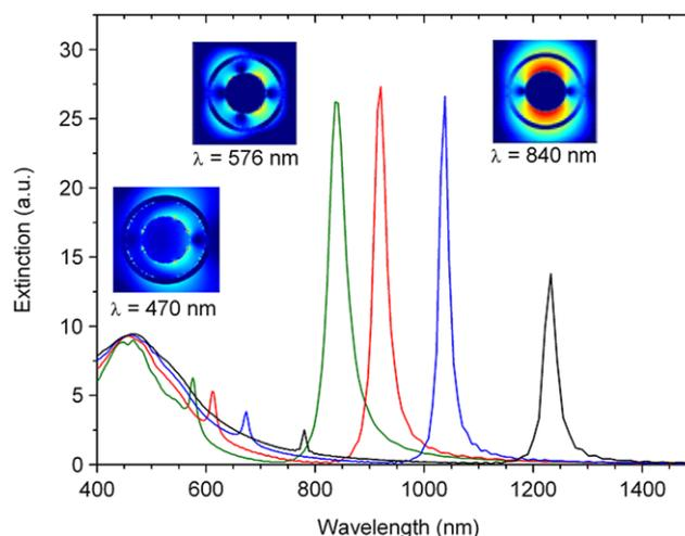
**Fig. 3** Extinction spectra for concentric MNS with  $R_2 = 66$  nm and  $R_3 = 75$  nm as a function of  $R_1$  for:  $R_1 = 40$  nm (green), 45 nm (red), 50 nm (blue) and 55 nm (black). Insets: electric field intensity plots for 40–66–75 nm MNS (green curve). The narrow and broad dipole resonances can be seen, as well as the quadrupole Fano resonance
